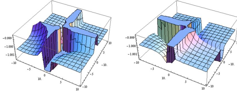
FIGURE 1. Solitary wave solutions of (3.1),  $u_1(x, t)$ ,  $u_2(x, t)$  are shown at  $a = 10$  and  $\alpha = 0.25$ .
